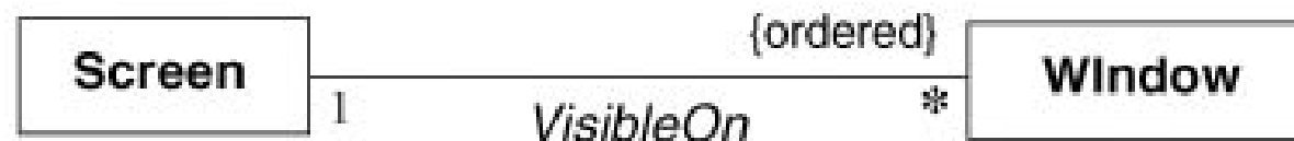
Figure 3.15 Ordering the objects for an association end. Ordering sometimes occurs for "many" multiplicity.
